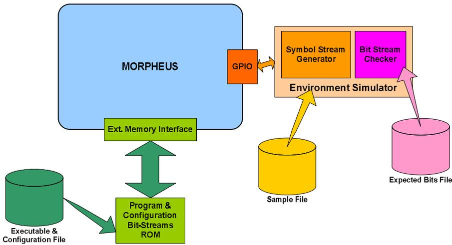
Figure 17-11. The Simulation environment for the wireless PHY segment on MORPHEUS
