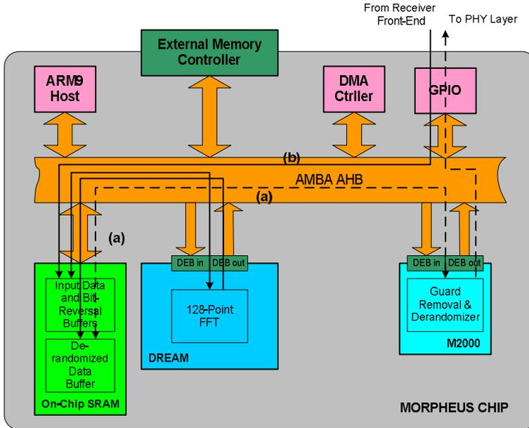
Figure 17-10. Illustration of the application mapping onto MORPHEUS
