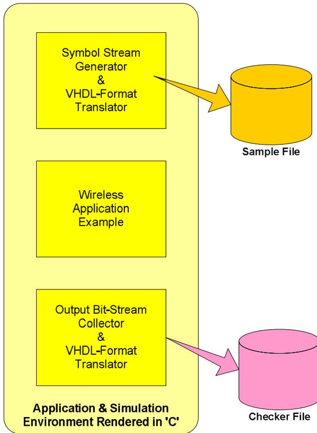
Figure 17-9. Outline of the application template/test-data generator implemented in 'C'
